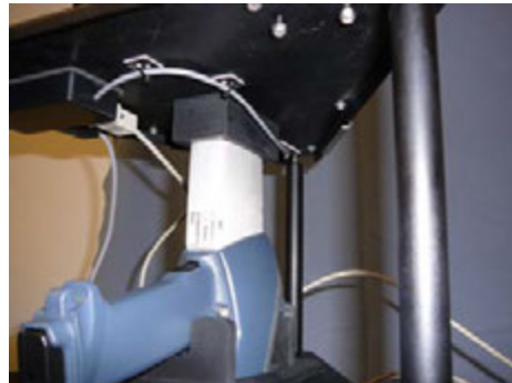
Figure 2.18. Mounting Upper Stand onto Test Stand.
