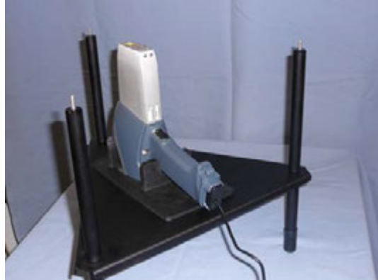
Figure 2.16. Analyzer Mounted in Cradle
