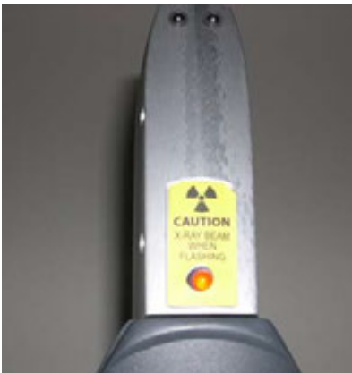
Figure 3.5. Probe light and labeling. When the light is on continuously, the x-ray tube is receiving minimal power and it is producing a minimum level of x-rays. The shutter is also closed so there is no radiation exposure to the operator or bystanders.
