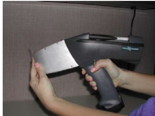
Figure 4.4 Extreme example of incorrect usage. An operator should NEVER hold small samples by hand
