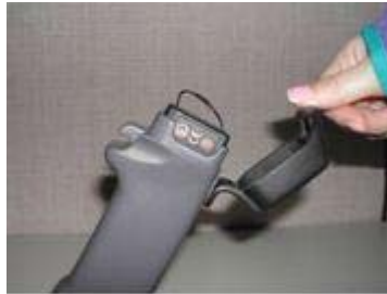
Figure 2.2a. Instrument handle. Pull the rubber latch and lift door. Reach into opening and remove battery.
