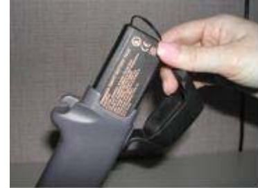
Figure 2.2b Insert new battery into opening.
