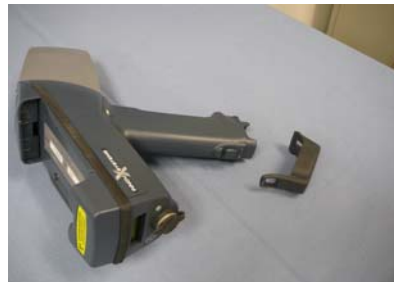
Figure 2.14. Rubber Boot Removed from Handle
