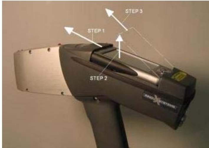
Figure 2.4. Removing the iPAQ from the analyzer.
