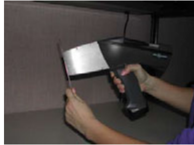
Figure 3.3. Incorrect Usage. While the dose to the operator's fingers/hand is negligible, testing this way sets a poor safety example for other operators, possibly encouraging other unsafe usage. Innov-X strongly recommends against this type of testing.
