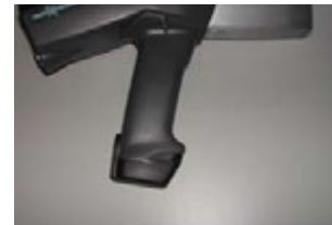
Figure 3.1 Handle of analyzer. Trigger is located at top of handle.
