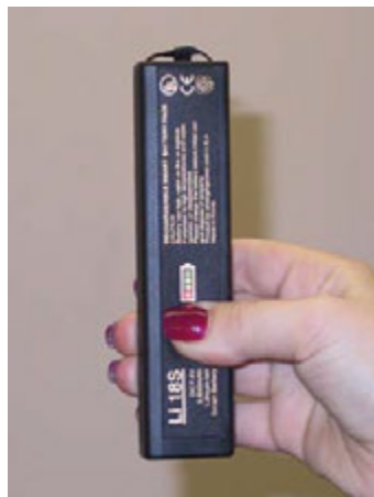
Two, Li-ion batteries (one shown).
