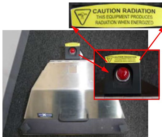
Figure 2.24 Top View of Test Stand (P/N A010-C) Shows Canadian Radiation Caution Label
