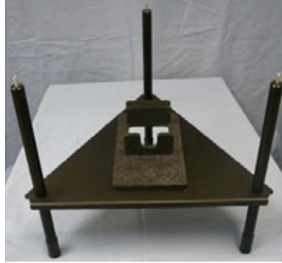
Figure 2.13. Mounting Long Legs onto Lower Stand.
