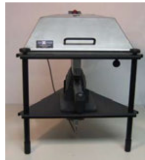
Figure 2.6. Assembled Test Stand: Analyzer Configured for iPAQ. (P/N A010)
