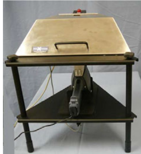
Figure 2.11. Assembled Test Stand: Alpha instrument configured for PC (P/N A010-C)
