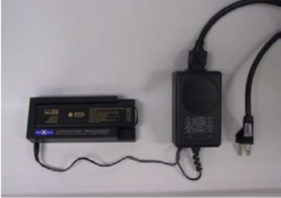
Battery charger and an AC adaptor. Battery shown mounted in charging system.
