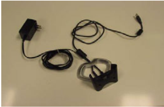
iPAQ cradle and AC adaptor. The cradle is used to connect the iPAQ to a PC for downloading data and reports.
