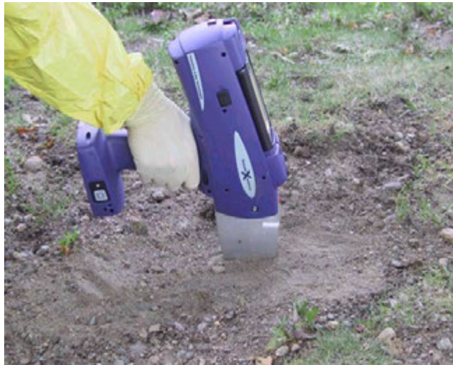
Figure 1. Use of a field portable XRF for in-situ soil testing.
