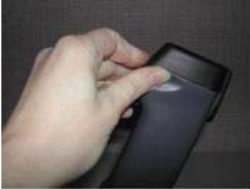
Figure 2.2a. Instrument handle. Pull the rubber latch and lift door. Reach into opening and remove battery.
